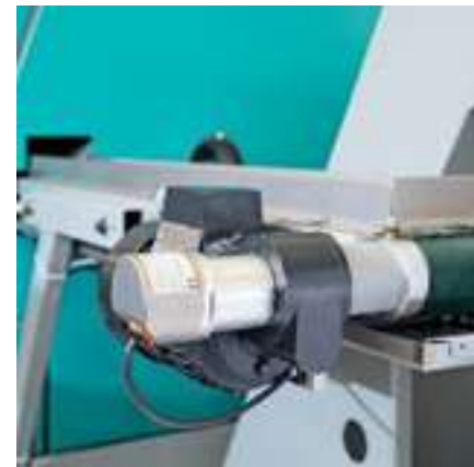
ifm's programmable incremental encoders allow you to select resolution and output type via IO-Link.
