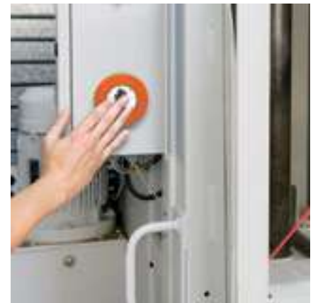
Mechanical machine start/stop buttons are susceptible to wear and tear. ifm's KT Series touch sensitive sensors operate without wear because they react to light contact for actuation and therefore provide a long life-in-application.
