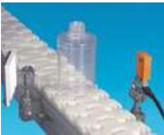
OJ sensor uses a reflector to detect plastic bottles on a conveyor.
