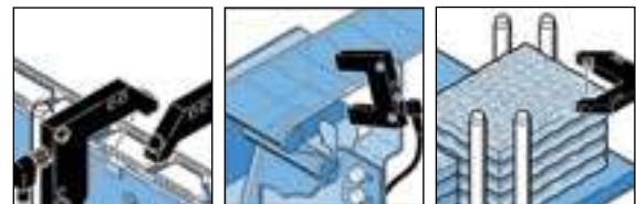
Detection of legs on integrated circuits
