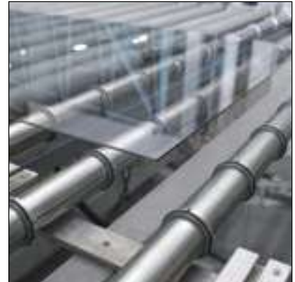
ifm's ultrasonic sensors detect targets regardless of their color, transparency or surface reflectivity.
