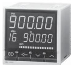
High-resolution inputs with a sampling cycle of 0.025 seconds and PID constants that can be set in increments of 0.01 seconds enable this controller to control process quantities that change rapidly. A strain gauge type pressure sensor can be directly connected.
